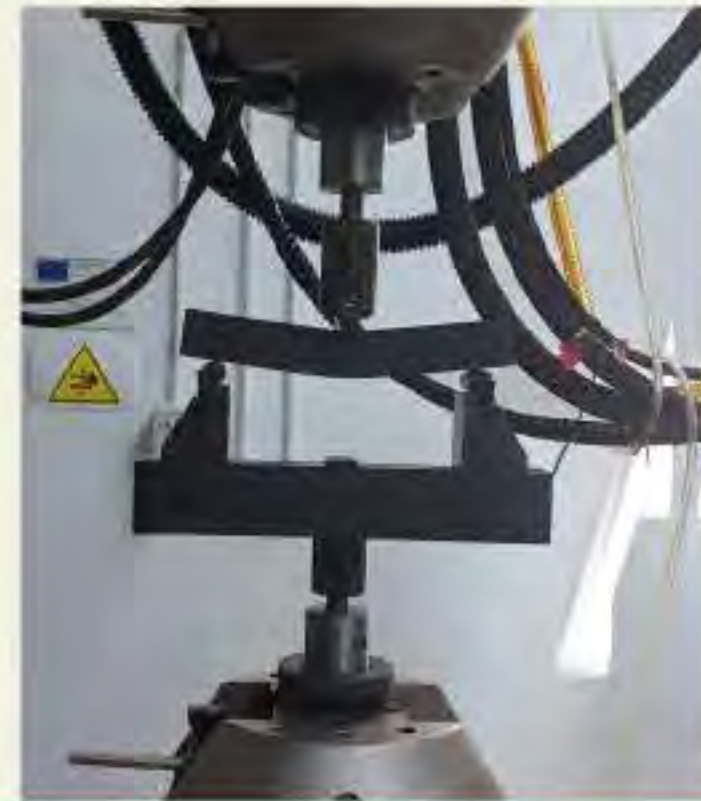
The specimen during and after bending test
