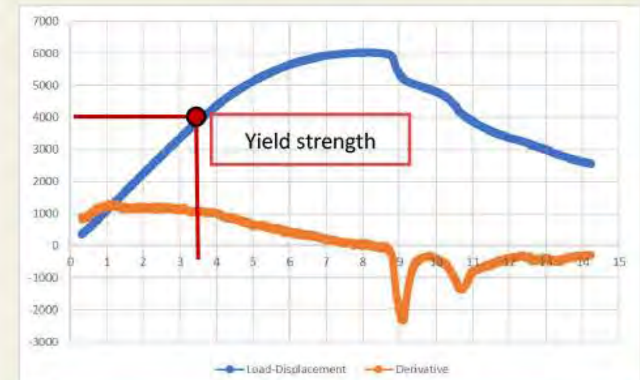
Load-displacement curve and its derivative (moving average)
