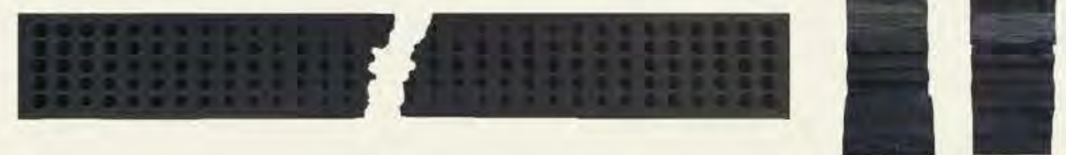
The broken specimen after 3-point bending test
