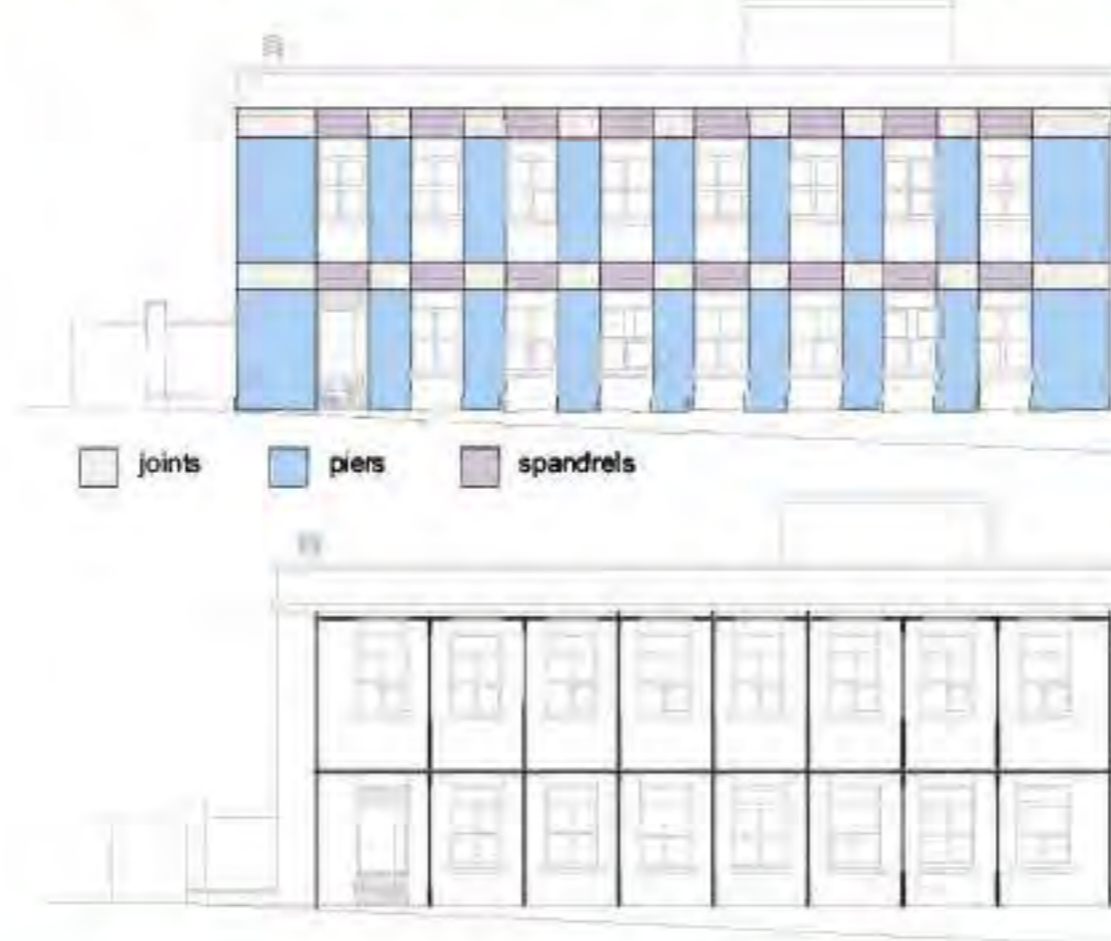
Numerical analyses are developed by a equivalent frame model and are conducted trough SAP2000 software.
