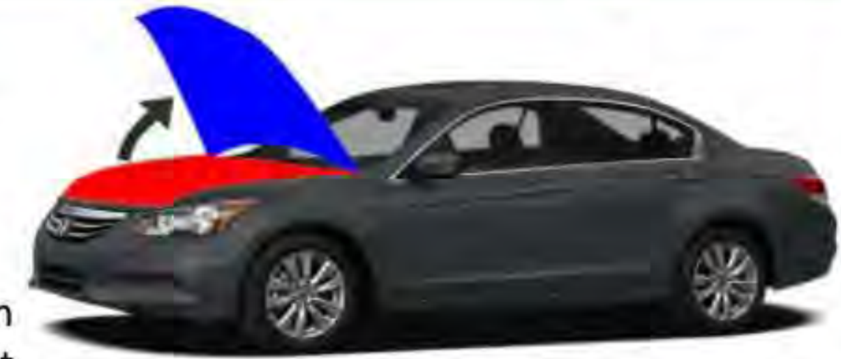
Figure 5: Rigid rotation to open the bonnet: SP in red, TP in blue
