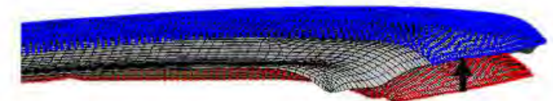
Figure 6: Surface targeting. SP from the starting mesh are moved towards the TP of the CS15 surface
